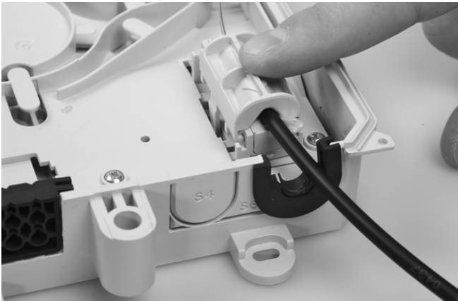
3.10 Install the cable holder into the box on the lowest position (adjust the position depending on the cable diameter).
