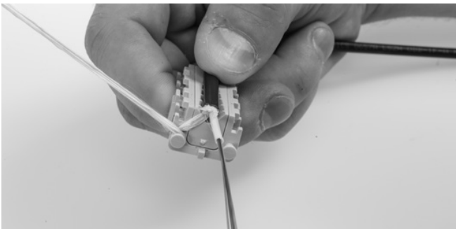
3.6 Install the feeder cable into the cable holder.
