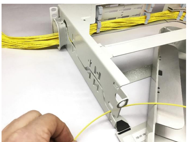
10.4.5 Feed the jumpers to the subunits. If the MFPS shelf is back mounted, you can use the side slit of the panel to feed the jumpers to the subunits.
