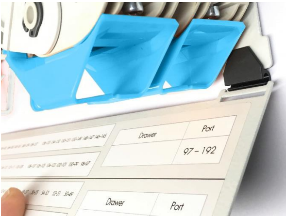
10.1.3 Take the front cover, place it into the slot of the hinges by an angle of 45°, push until the cover is fixed. Repeat on the other side.
