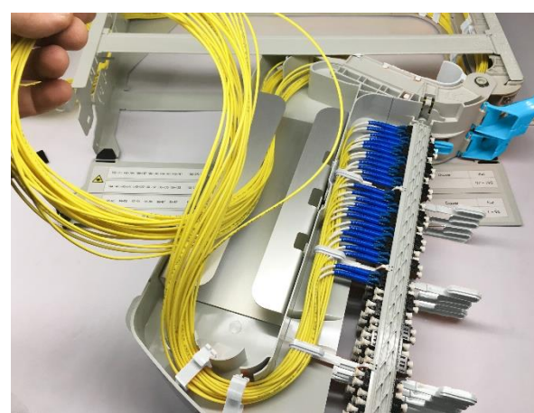
10.4.8 Make all patches first before storing the over length.
