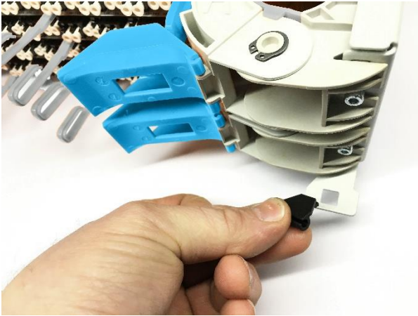
10.1.1 Install the hinge on right side of the shelf by first inserting the narrow end of the hinge into the hinge slot and then snap it into place.
